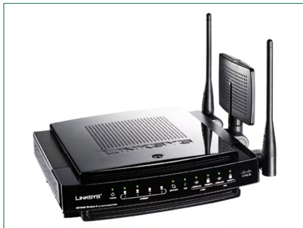
Three antennas! A dual-band WiFi router to the 802.11n MIMO standard. (With kind permission from Linksys).
