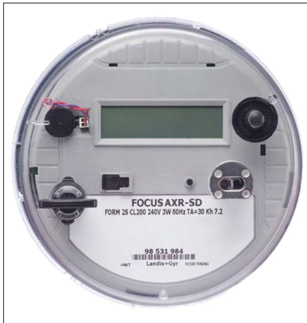
The FOCUS AXSD is an advanced ZigBee meter/circuit-breaker that forms part of an intelligent network (Smart Grid). (With kind permission from Landis + Gyr) (With kind permission from Maxim).
