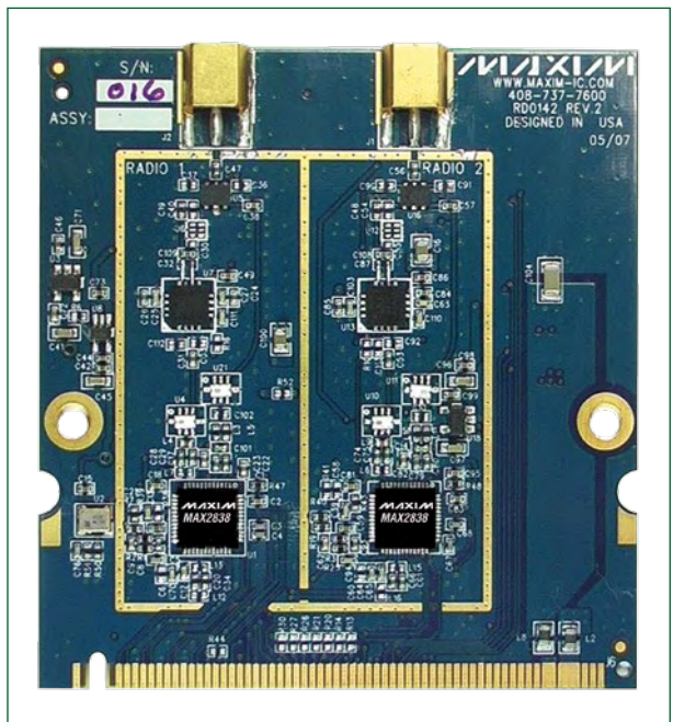
WiMAX reference development card using the MAX2838.
