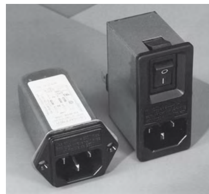
Standard mains filters built into a mains entry together with an on/off switch. The metal shell must be in firm contact with the enclosure.
