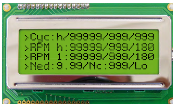
Figure 13. On this screen, you can define just how the automatic running-in is performed.
