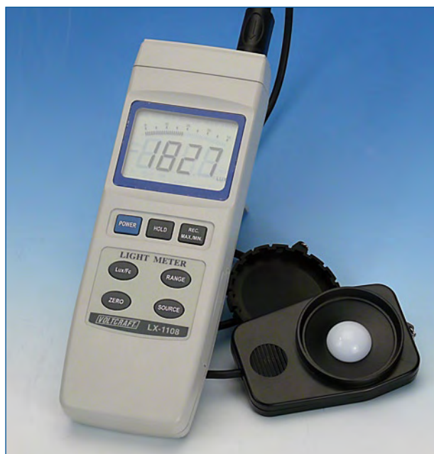
Figure 2. A light meter calibrated in lux is indispensable for measuring light intensity. For our measurements, we used a Voltcraft LX-1108 provided by Conrad Netherlands.
