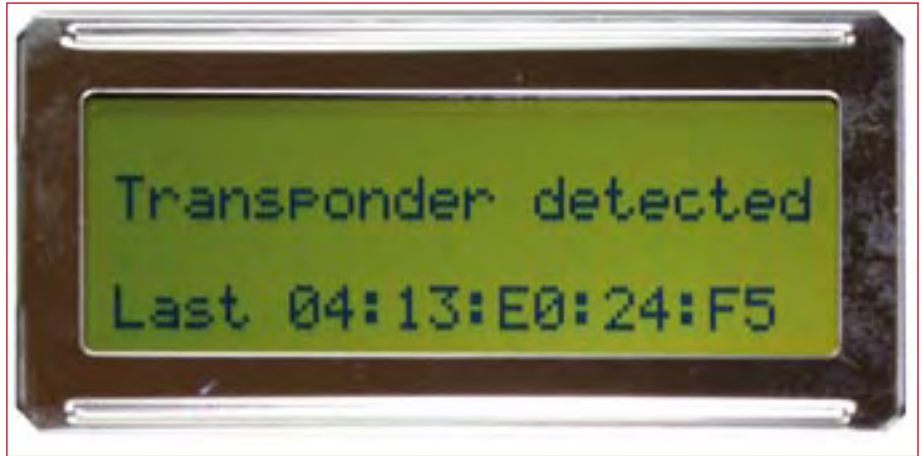
Figure 11. When a RFID tag is recognised, the data read from the tag is shown on the LC display.
