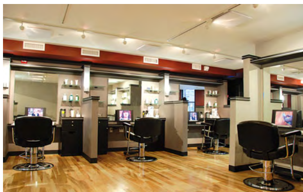
Figure 8. Hairdresser high-tech. In the ceiling there are panels that form part of the 'Audio Spotlight' system by American manufacturer Holosonics. The panels create an ultrasound field using a vibrating metal-polymer hybrid film.
