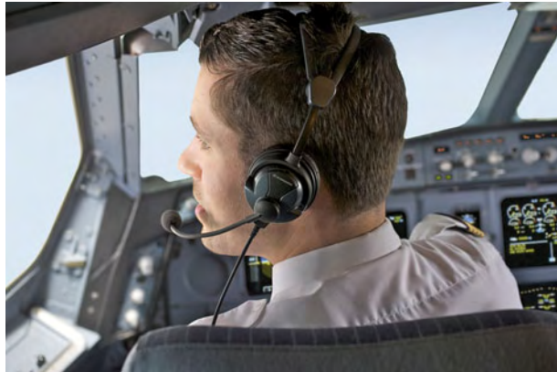
Figure 10. Anti-sound headphones by Sennheiser. The 'NoiseGuard' range uses analogue circuitry, which the manufacturer claims has benefits in terms of cost and speed.
