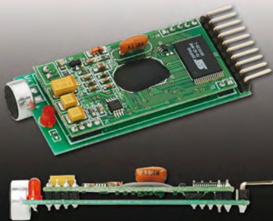
Say It Module (#30080) Provides voice recognition for built-in pre-programmed commands and up to 32 user defined commands! Good for robots, home automation, and more.
