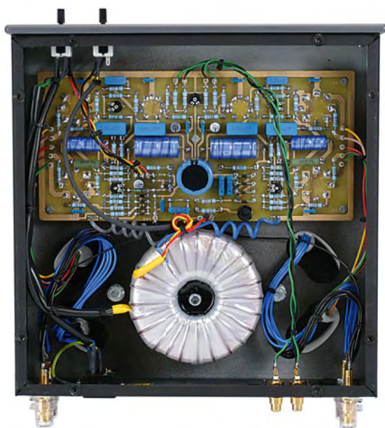
Figure 4. Bottom view of the power amplifier. All of the circuitry, including the valve sockets, is located on a single PCB.
