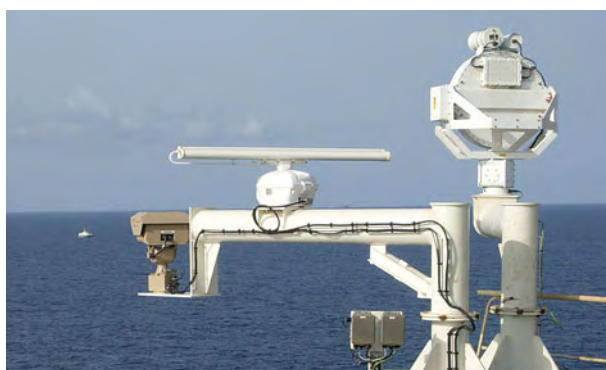
Figure 9. The LRAD (Long Range Acoustic Device) is the circular object towards the top right of the picture. The loudspeaker arrangement creates sound at levels of up to 150 dB, enough even to ward off pirates!
