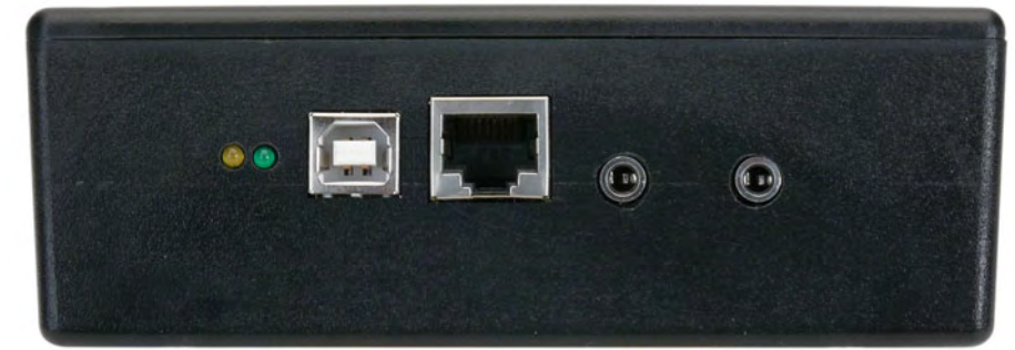
Figure 2. The attenuator unit. From left to right: the yellow LED indicates when communication with the PC takes place, the green LED shows when the supply voltage is present. Next to that is the USB connector, the RJ45 connector for the push button box, the signal input and finally the connector for the headphones.
