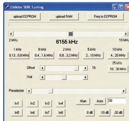
Figure 6. The tuning software now also drives the preselector.
