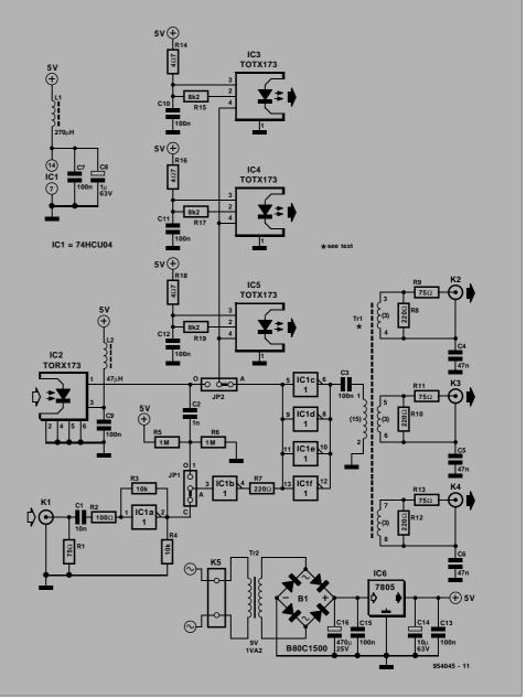
about half the core, while the secondary windings of three turns each are distributed over the remainder. All windings are made from 0.5-mm dia (24 SWG) enamelled copper wire.
