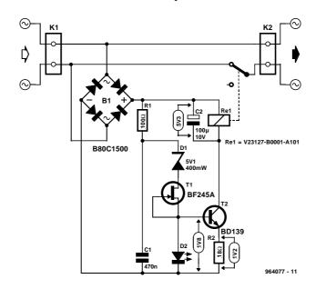
testing with music or white noise (13 W off, 5 W on). Network R1-C1 is a rudimentary peak detector which helps to improve the response of the circuit to noise.
