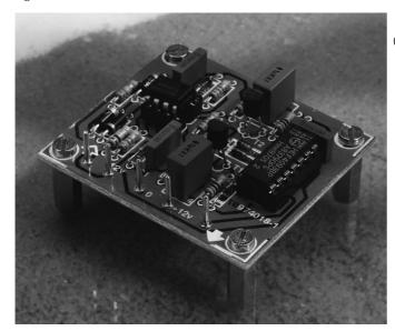
The signal from the amplifier is applied to the sensor via  $R_{10}$ . Its level is limited by diodes  $D_2-D_5$ . The trip levels of comparators  $IC_{2a}-IC_{2b}$  are set to + 600 mV and -600 mV by  $R_2$ - $D_6$  and  $R_3$ - $D_1$  respectively. This means that the output of  $IC_{2a}$  goes high when the input voltage is higher than + 600 mV and that of  $IC_{2b}$  when the input voltage is lower than -600 mV.
