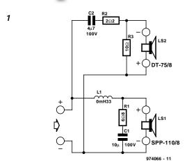
In this design of a simple loudspeaker enclosure an attempt has been made to achieve a reasonably good quality with a minimum of material. In spite of inexpensive drivers, this aim was met.
