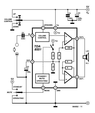
to 40 dB (low volume), so the gain of the total amplifier is then -20 dB. Some positive pulses have to be applied to the UP/DOWN pin to achieve listening volume. The graph shows the THD as a function of output power. The maximum quiescent current consumption of the amplifier is specified at 10 mA, to which should be added the current resulting from the output offset voltage divided by the load impedance.
