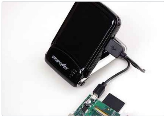
◀ A portable power pack will keep your Pi running when it's away from the mains
