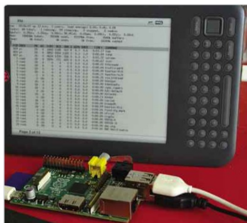
▼ Use your Kindle as a screen for the Raspberry Pi, with KindleBerry Pi
