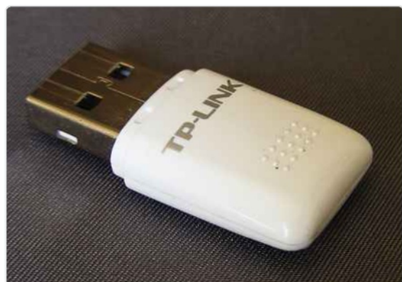
▲ A USB Wi-Fi adapter is a handy way to network the Pi
