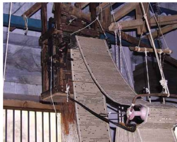
▲ Programming is nothing new - Jacquard's loom was an early example of how to create a sequence of commands
