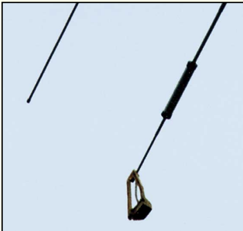
Once upon a time, Dave, K6JOX, and John, KE6PID, were doing some antenna work at ground level thanks to Dave's tilt-over tower. With their task completed, Dave worked the crank to raise the tower while John watched closely to make sure the tip of the Yagi's driven element cleared the edge of Dave's house on its way up. Unfortunately, neither noticed that the opposite side of the Yagi had firmly snagged Dave's lawn sprinkler!
