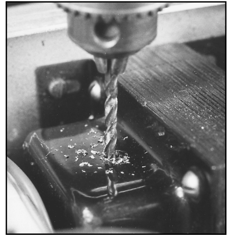
Figure 3—A hole being drilled in a Heathkit SB-220 transformer during early testing.
