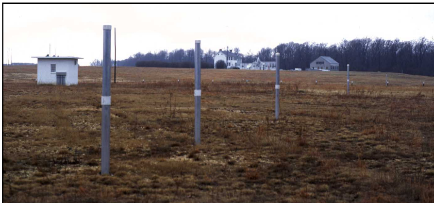
Six-foot tall poles like these—each an active antenna—have replaced rhombics and Yagis for HF monitoring at FCC facilities. These are part of an interferometric array.
