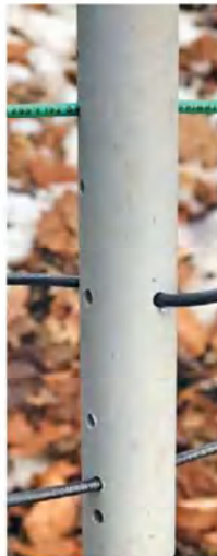
Figure 6 — The long PVC spacer with holes drilled 2 inches apart at slight angles to each other to minimize slipping on the wires.
