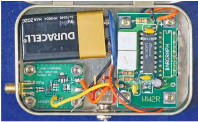
Figure 3 — An inexpensive power meter capable of operation on frequencies from 1 MHz to 10 GHz. The AD8317 module used is the second from the right in Figure 1. The LED indicator is displaying -30 dBm ( 1 \mu\text{W} ) at 3.4 GHz.
