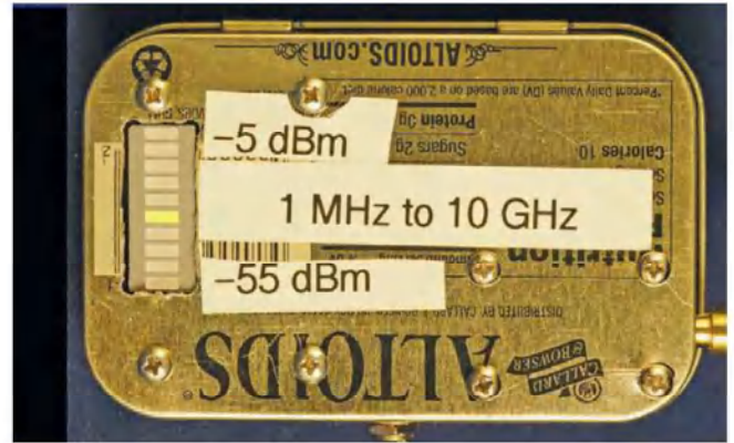
Figure 3 — An inexpensive power meter capable of operation on frequencies from 1 MHz to 10 GHz. The AD8317 module used is the second from the right in Figure 1. The LED indicator is displaying -30 dBm ( 1 \mu\text{W} ) at 3.4 GHz.
