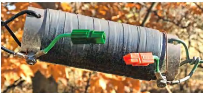
Figure 5 — The 80-meter loading coil with disconnected jumpers. The coil is wrapped with electrical tape to stabilize and weather-proof the magnet wire. It's also painted gray for aesthetics. Note the method for attaching the coil form to the 40-meter (on the left) and 80-meter (on the right) wires.
