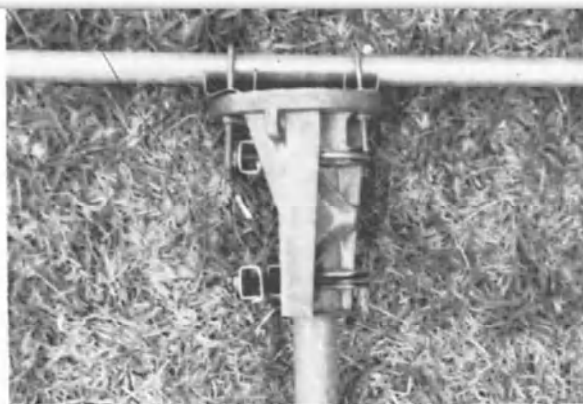
Fig. 2 — The bottom section of a CDE Ham-M rotor can be adapted to serve as a boom-to-mast bracket.
