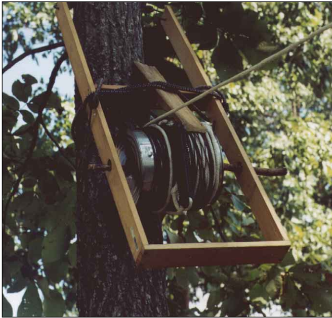
The wire antenna and tie ropes can be kept under control with this simple homebrew device. The spool is a coffee can and the “drag” can be made from a piece of scrap wood and a bungee cord.
