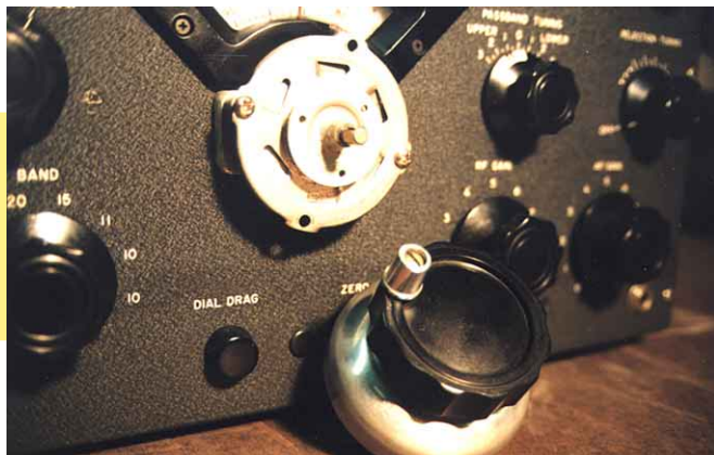
Detail of the homemade gear reduction assembly and hand-milled knob skirt for K’s homebrew 75A-4.
