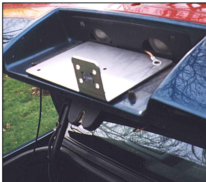
The main plate of the TM-1 is ready for installation. Note the ground strap in the upper corner.
