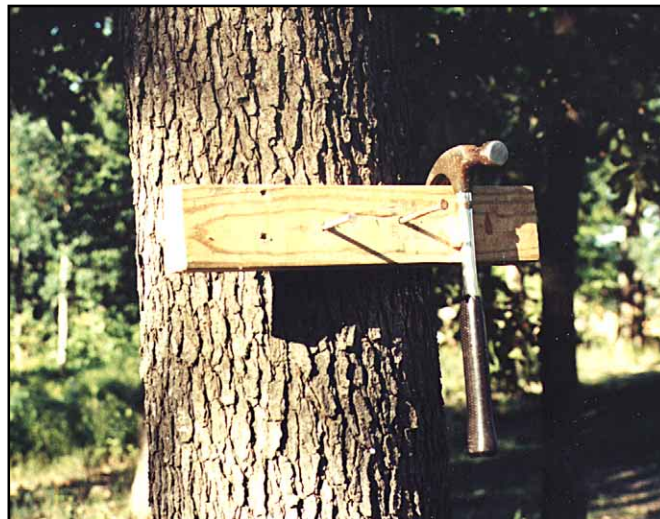
A handy climbing cleat. Drive 5-inch nails into the trunk through holes drilled in a 2 × 4.
