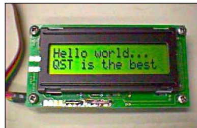
Figure B—These simple-to-use character-based displays really give a professional appearance to our projects. They can be programmed serially themselves, or connected directly to a PIC through six I/O pins.
