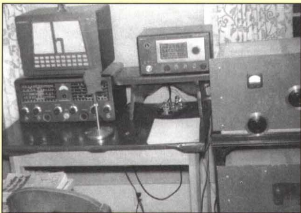
W9JTN, 1952, with SX-71, HT-18, Pair of 814s— about the same Power as a modern transceiver. 40 meter dipole
