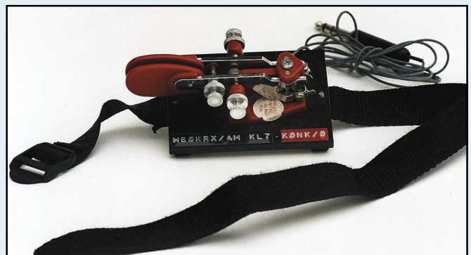
The paddle I use was originally configured to support HF CW operation while flying a single-engine airplane on a trip to Alaska. It has since become standard equipment on backpacking trips. The paddle is a Ham-Key model HK-2 (no longer manufactured) mounted on a plastic base. A nylon strap comes off the back and an elastic strap comes out the front to hold it securely to my leg. Today, a handy backpacking paddle that includes a leg strap is available from Paddlette Company, PO Box 6036, Edmonds, WA 98026. Also, Winterook Products carries small paddles and keys.
