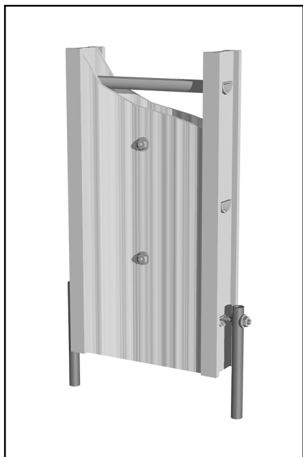
Figure 1—WOMLG's plywood sandwich prevents unwanted climbers from ascending the extension-ladder antenna support.
