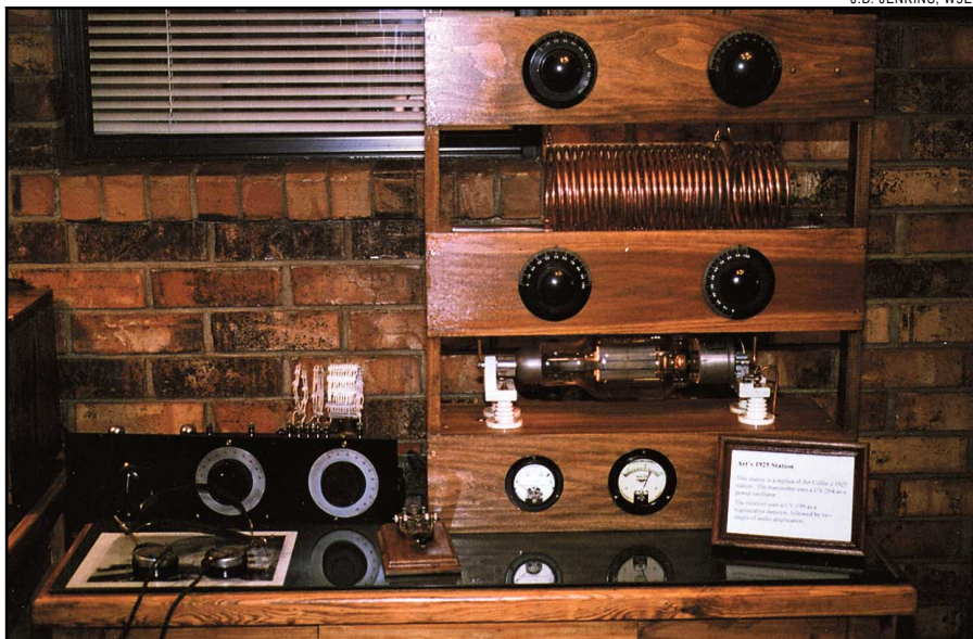
W5EU's hand-made replicas of an Arthur Collins transmitter and receiver.
