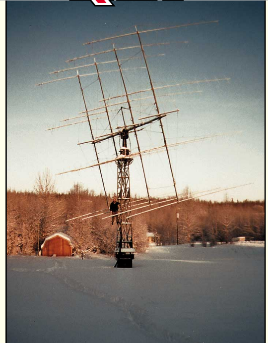
Yes, they do moonbounce in Alaska—even in the dead of winter. Look closely and you'll see Chris Hazlitt, KL7FB, standing on the tower that supports his impressive moonbounce antenna array near Palmer, Alaska.
