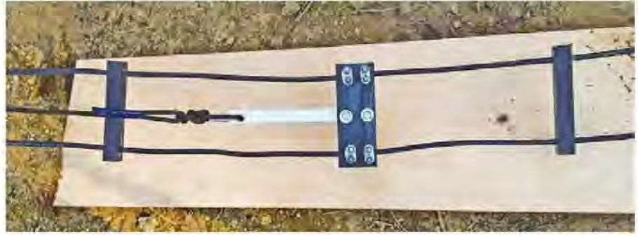
An aluminum U channel connects the assembly to a rope.
