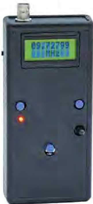
Figure 11 — The HeckKits 50 \Omega Bridge/Frequency Counter is mounted in a plastic case with a two-line by eight-character LCD.
