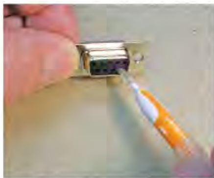
Figure 4 — Sockets on small connectors, like the DB9 shown here, can be cleared of dirt and contaminants with an interdental brush. [Henry Boze, N4HB, photo]
