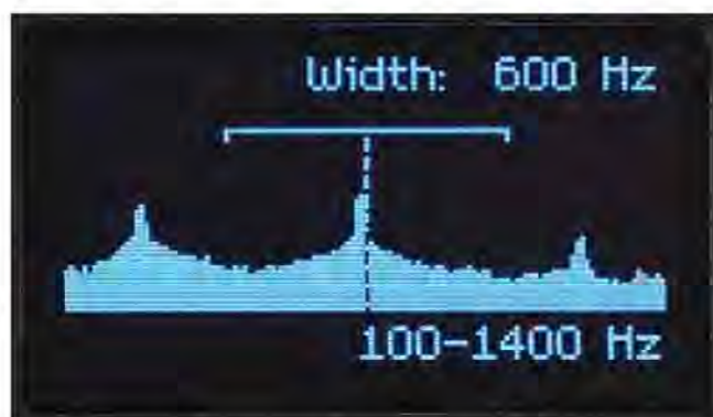
Figure 7 — The Wolfwave set up for a 600 Hz CW filter with a center frequency of 650 Hz.
