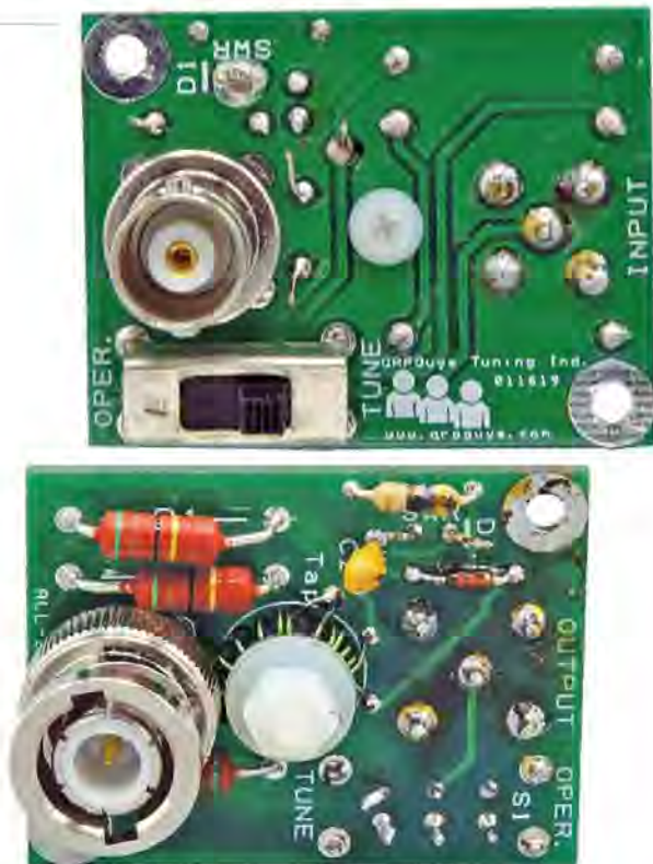
Figure 10 — The QRPGuys LED Tuning Indicator requires no external power source. The input (male) BNC connector is shown here on the component side of the board, with the output BNC connector, indicator LED, and BYPASS switch on the other side. The board is intended to mount directly on the antenna jack of the companion QRP transceiver.
