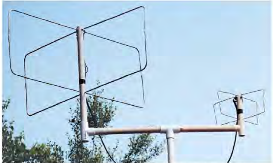
Figure 1 — L.B. Cebik's, W4RNL, dual-Moxon phased array antennas for 2-meter and 70-centimeter satellite work.
