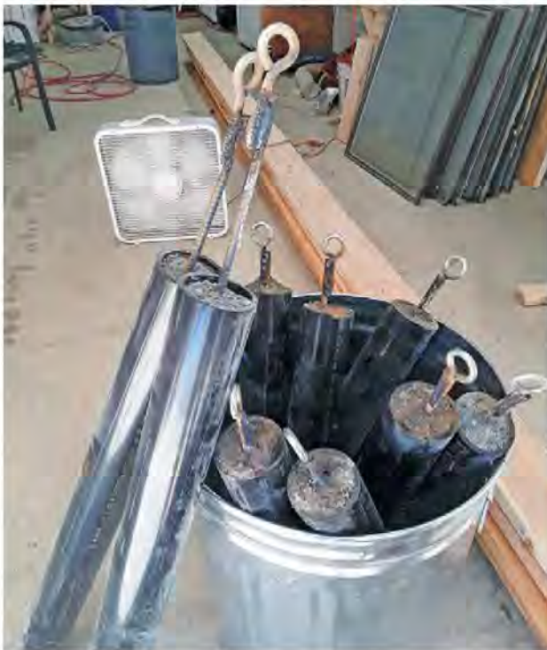
A collection of counterweights made from concrete poured inside 3-inch standard ABS plastic plumbing pipes.
