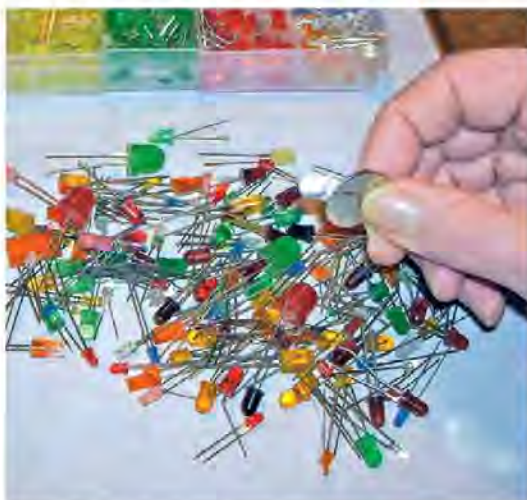
Figure 1 — Sliding a 3.6 V battery between the leads of an LED provides an easy method to test whether the LEDs are working. [William Gerhold, K2WH, photo]
