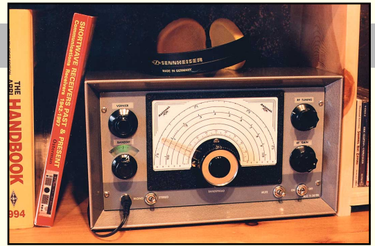
Binaural beauty. If you read the article by Rick Campbell, KK7B, in the March 1999 QST , you know about his fascinating binaural I-Q receiver design (“A Binaural I-Q Receiver,” page 44). Here is the same receiver in an attractive homebrewed cabinet. Rick crafted the enclosure using items (such as the National dial) scavenged from hamfest flea markets.
