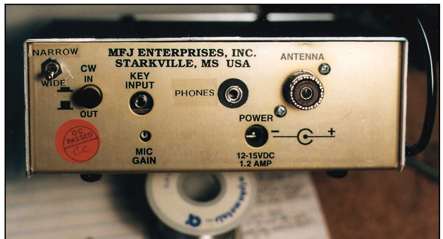
Figure 2—A rear view of the transceiver shows the new CW-filter switch at the upper left and the new headphone jack at the center. The dark circuit around the PHONES jack is a fiber shoulder washer to insulate the jack from the cabinet.
