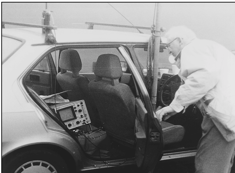
Derek Atter, G3GRO, presses the CALL button on the mobile radio in the front of the car. The IC-2E hand-held on the roof is monitoring the transmitted signal and the IC-2E beneath the oscilloscope is receiving the signal from the repeater.
