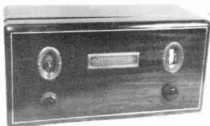
RADIOLA 16 AR-924 6 TUBE RECEIVER UX 201As 1927
