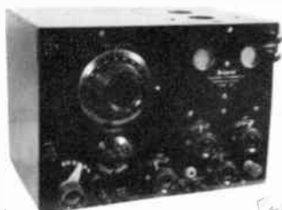
Federal 57 FEDERAL 57 RECEIVER SINGLE TUNED RECEIVER 1 STAGE R.F. DET. 2 STAGE AUDIO 1922 S.P. $98.00
