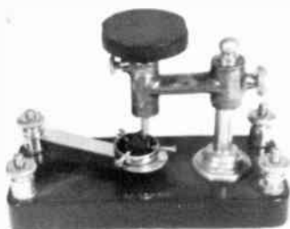
MURDOCK SILICON DETECTOR WITH CONDENSOR 1913 $4.50
