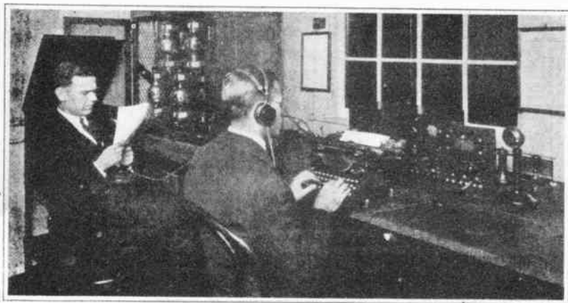
The "announcer" of a radio-phone broadcasting station, and the receiving operator. The announcer speaks into the microphone transmitter which he holds in his hand. Alongside of him is the radio-phone transmitting apparatus, with the vacuum tubes for generating and modulating the radio waves. This is WJZ, the Newark radiophone.
