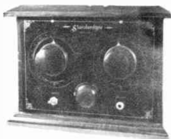
STANDARDYNE THREE TUBE SET USING MULTIVALVE TUBE THREE TUBES IN ONE 1925
