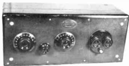
ATWATER KENT MODEL 20 5 TUBE T.R.F. 1924 $80.00
