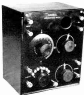
SIGNAL SINGLE CIRCUIT REGEN. ONE TUBE $25.00
