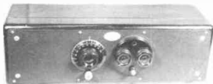
ATWATER KENT MODEL 30 6 TUBE T.R.F. 1924 $85.00 combined ant.
