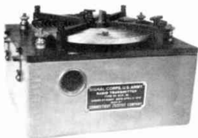
U. S. ARMY SPARK TRANSMITTER FIRST TYPE USED IN AIRPLANES 1918
