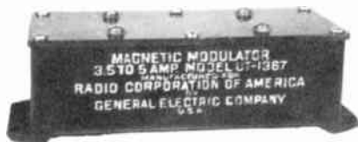
RCA MAGNETIC MODULATOR USED IN ANT. CIRCUIT 1922
