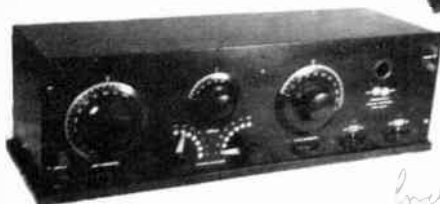
Grebe 1-7 Radio GREBE CR-8 ONE TUBE REGEN. 150 TO 1,000 M. 1921 $80.00 Grebe 1-5 R. d.
