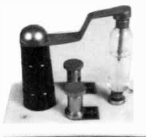
ELECTRO IMPORTING CO. RADIOSON ELECTROLYTIC DETECTOR, ABOUT 1914
