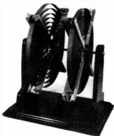
AMCO OSC. TRANS. 1 KW MADE FROM KIT ABOUT 1914
