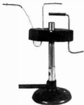
DEFOREST GAS FLAME DETECTOR FORERUNNER OF THE VACUUM TUBE REPLICA 1904
