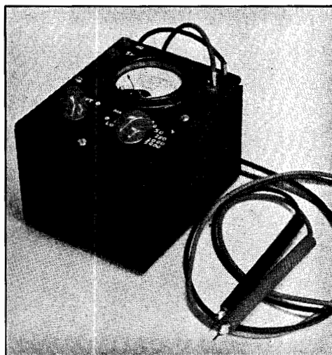
Fig. 1721 — The inexpensive multi-range volt-ohm-milliammeter is housed in a standard 3 x 4 x 5 metal cabinet. Ranges are marked with number dies, the impressions being filled with white ink. High-voltage test leads are available for use on the 5000-volt range.
