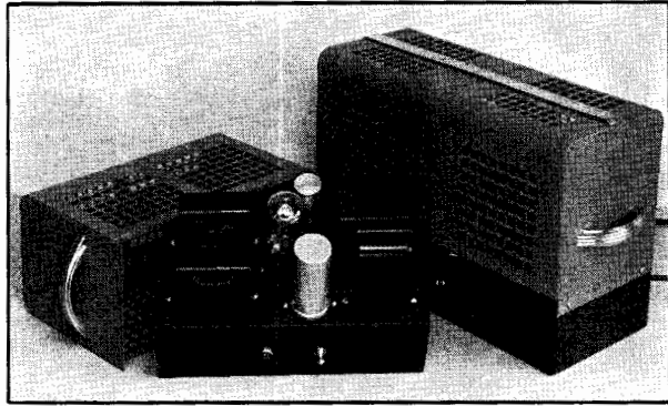
Fig. 1122 —Two typical receiver power supplies. The small 100 ma. supply is assembled on a chassis 5 in. by 10 in. by 3 in., while the larger 200-ma. supply is built on a chassis 6 in. by 14 in. by 3 in. The covers protect the equipment against damage and add to the appearance.
